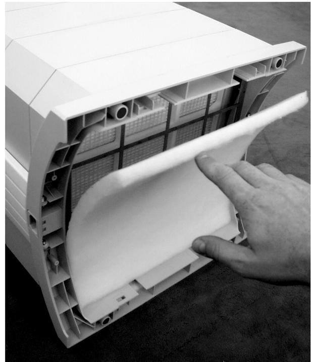
**4** The PF40 coarse dust filter pad has a rough, cottony side and a smooth side. Place the filter on top of the filter grille with the rough, cottony side facing outward. When properly installed the rough, cottony side will be facing the floor when the system is in its upright position.
