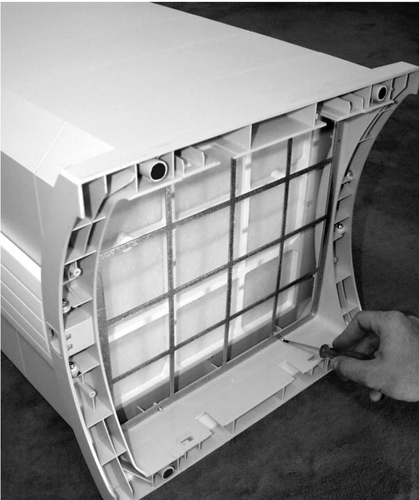
**3** Secure the filter grille with the eight Torx-screws and screw driver supplied with the installation kit. Ensure that all screws are tight, but be careful not to over-tighten the screws.
