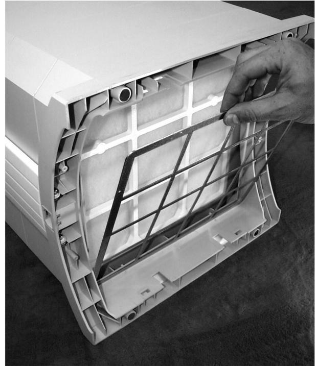
**2** Insert the filter grille with the holes along the edge into the base of the IQAir system.
